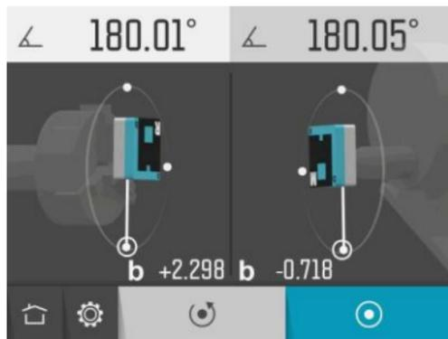
Rotate the sensors to the third measurement position, at the rotational angle  $180^\circ$ .
