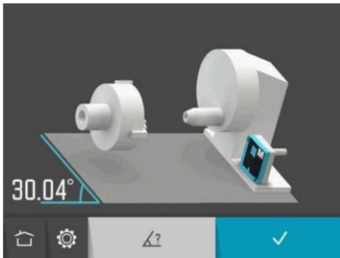
When measuring machine bed slant with the SM sensor, the angle value is displayed live.
