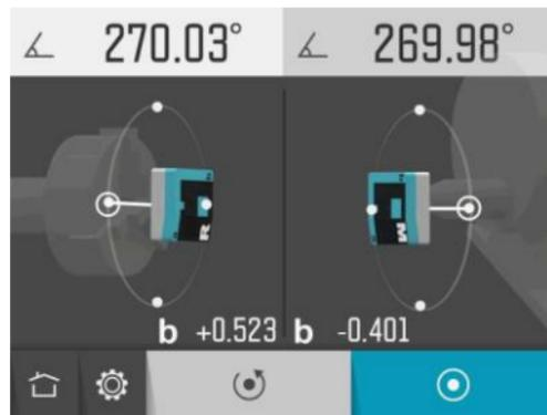
Rotate the sensors to the fourth measurement position, at the rotational angle  $270^\circ$ .
