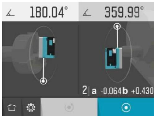
Move the tool holder with the SM sensor to the second measurement point.
