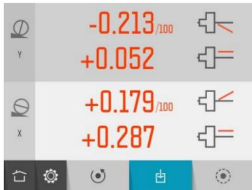
The measurement result screen displays angle and offset values in two directions, perpendicular to the machine bed slant and parallel to the machine bed slant.
