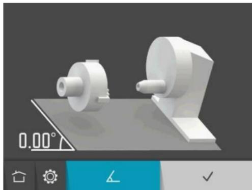
The machine bed slant is measured with the SM sensor.
