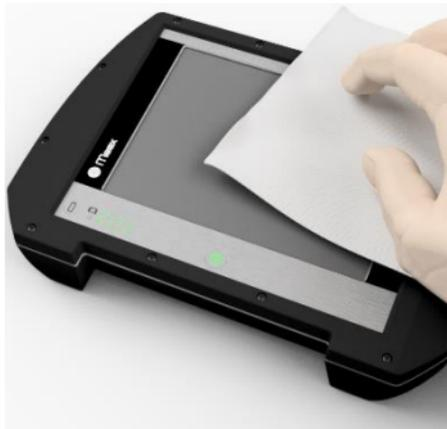
For the best possible function, the laser diode apertures, detector surfaces and connector terminals should be kept free from grease or dirt. The display unit should be kept clean and the screen surface protected from scratches.
