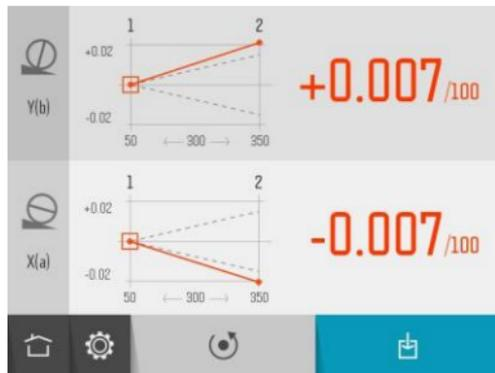
The measurement result screen displays angle values in two directions, perpendicular to the machine bed slant and parallel to the machine bed slant.
