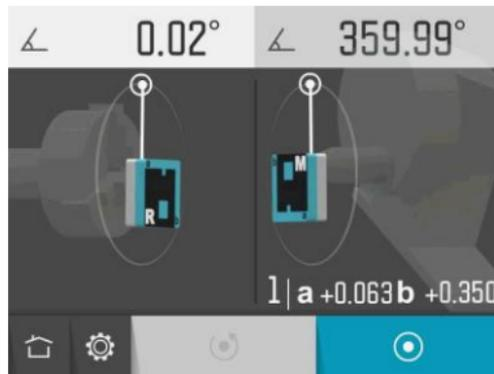
Place the tool holder with the SM sensor at the first measurement point and set the SM sensor at 0°.
