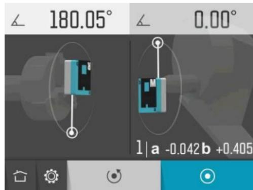
Rotate the SR sensor to the second measurement position at 180°.
