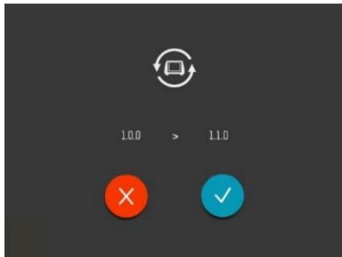
You can choose between exiting (and not upgrading) or installing the new software version. The version numbers of the existing and the new software are displayed above the icons.
