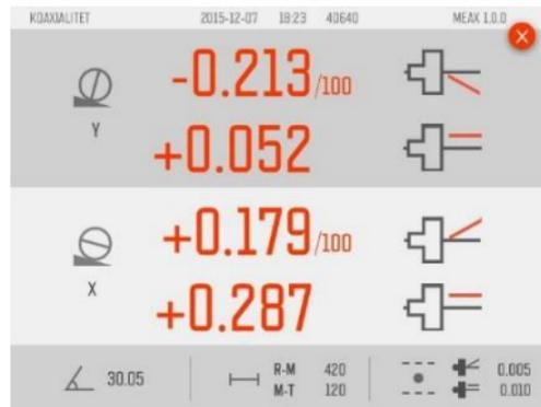
The screen displays measurement results, positions, distances, machine bed slant, tolerances, axes names, file name, date and time, serial number of the display unit, program and program version.
