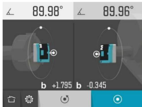
Rotate the sensors to the second measurement position, at the rotational angle  $90^\circ$ .
